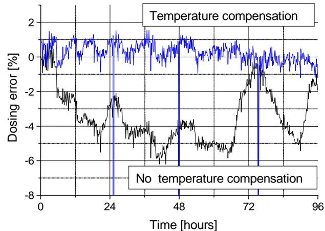
**Fig. 2:** Compensation for the dosing error of water due to temperature variation.
