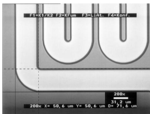
**Fig. 1:** The microchannel is located on the front side of a silicon chip and covered with a pyrex glass wafer (sectional microscope view, 200x).
