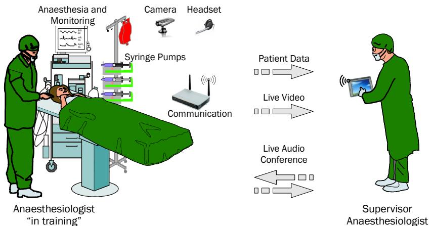
specific device drivers are implemented. For Audio/Video recording, off the shelf webcam equipment was used. Wireless data transmission is serviced by several IEEE 802.11b/g WLAN access points distributed in the OR-zone covering also wakeup room and staff area. The supervisor data terminal is a mobile DIN-A5 size tablet PC. Presentation of the data is styled after the accustomed layout of the monitoring system.
